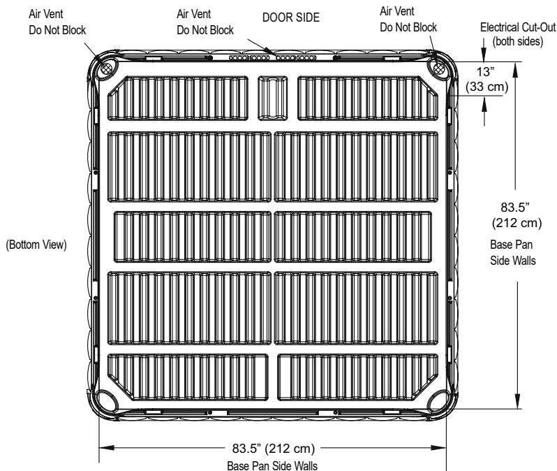
**NOTE: WATKINS WELLNESS** requires that the **GENEVA** and **NIAGARA** be installed on a minimum 4" thick reinforced concrete pad or structurally sound deck able to support the "dead weight" found in the spa specification chart.
