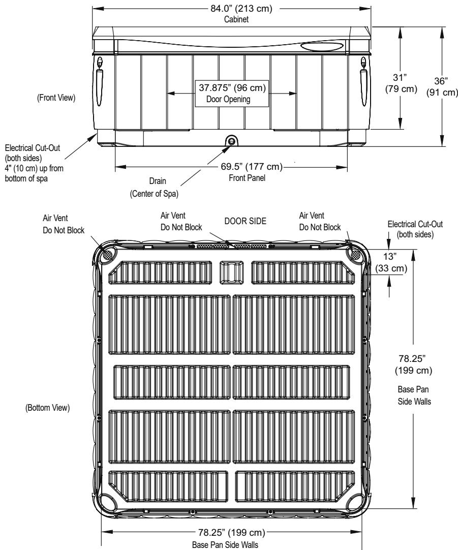
**NOTE: WATKINS WELLNESS** recommends that the **TAHITIAN** and **FLORENCE** be installed on a minimum 4" thick reinforced concrete pad or structurally sound deck able to support the "dead weight" found in the spa specification chart.
